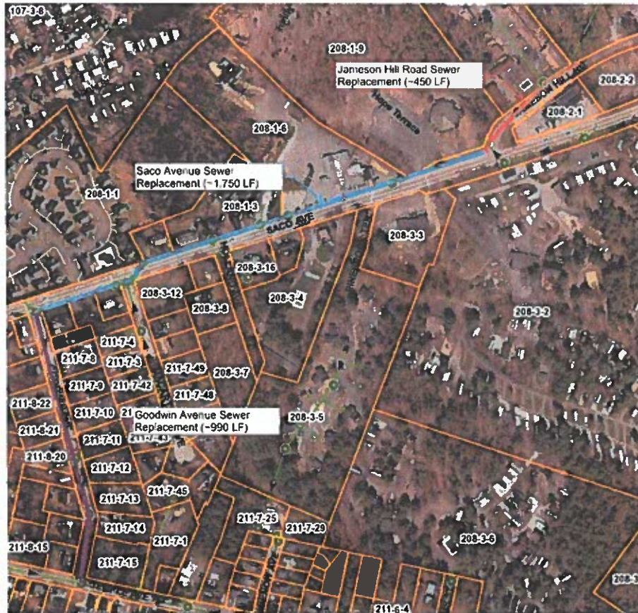
Figure 1 Limit of Sewer Replacement – Saco Area Sewer Improvements (reference Town of Old Orchard Beach GIS)
